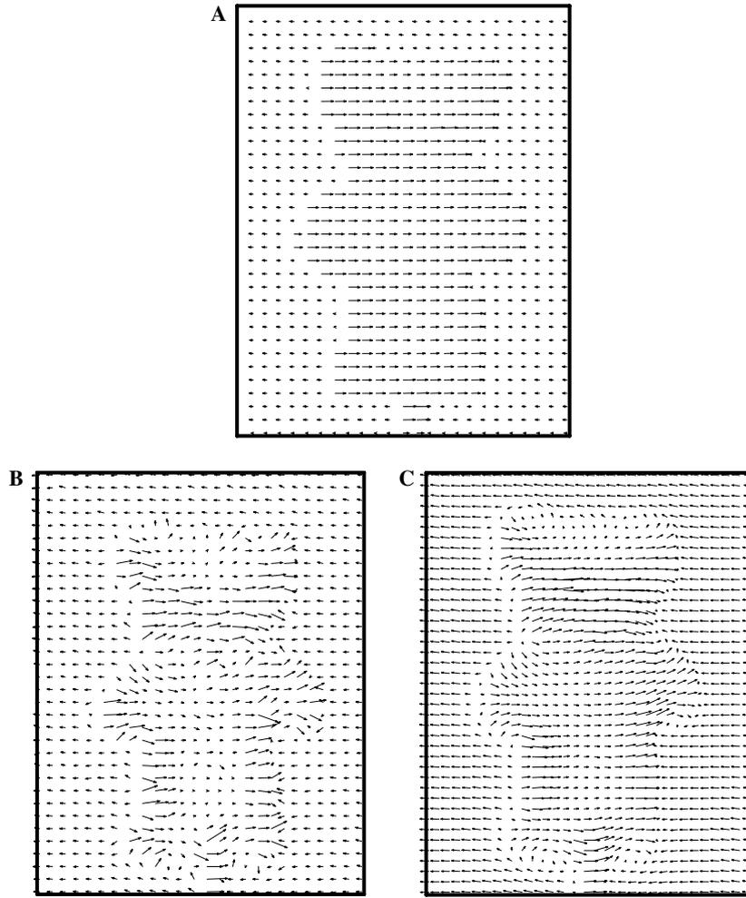
Fig. 8. Optical flow estimated by (A) this method; (B) the Horn-and- Schunck method; (C) the Aubert–Deriche–Kornprobst method.
