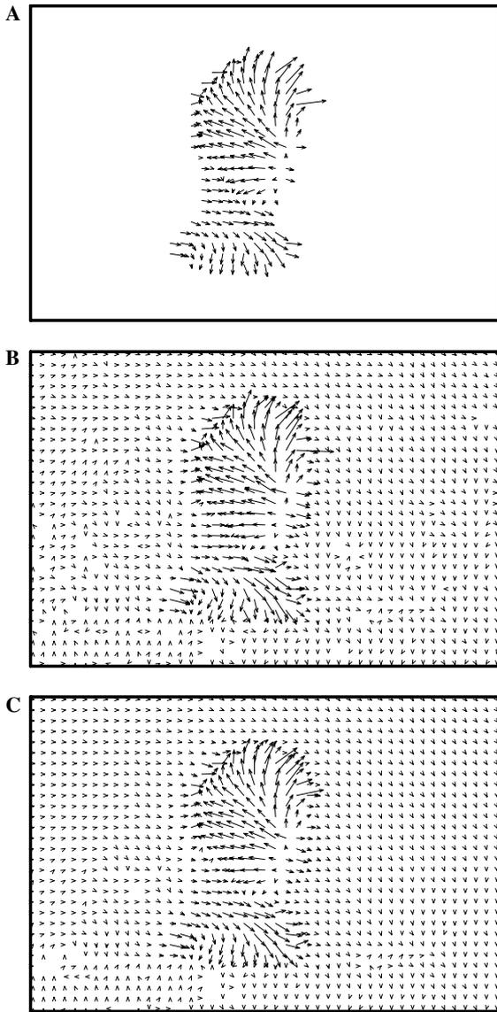
Fig. 5. Optical flow estimated by (A) this method; (B) the Horn-and-Schunck method; (C) the Aubert–Deriche–Kornprobst method.
