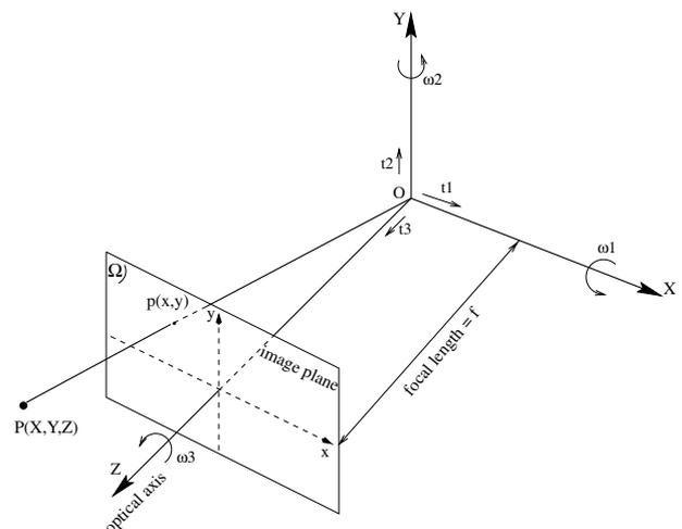
Fig. 1. The viewing system is modeled by an orthonormal coordinate system and central projection through the origin.
