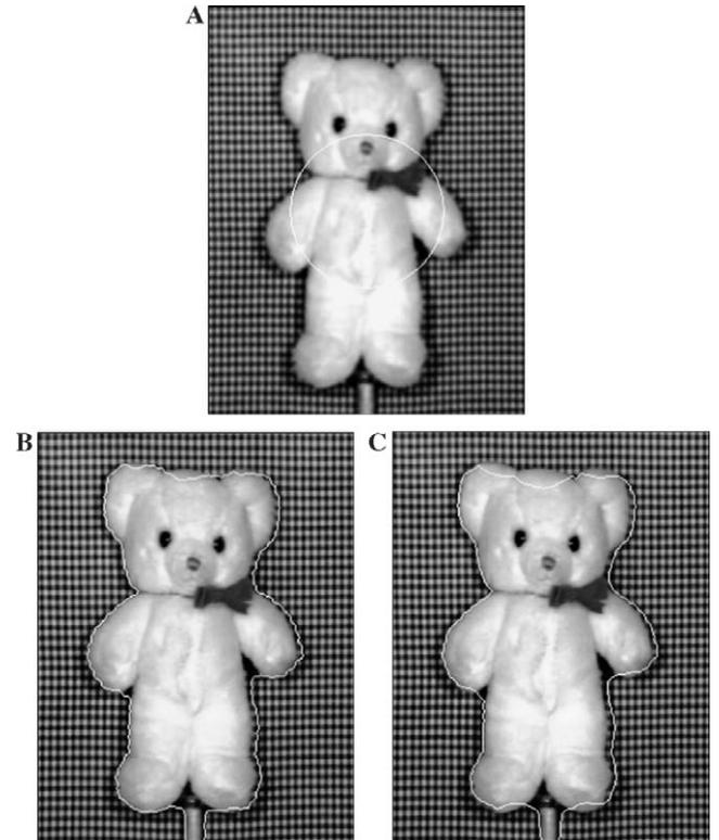
Fig. 6. (A) The first frame of *Teddy1* sequence and the initial level set; (B) the computed segmentation; (C) the segmentation without the 3D interpretation term.
